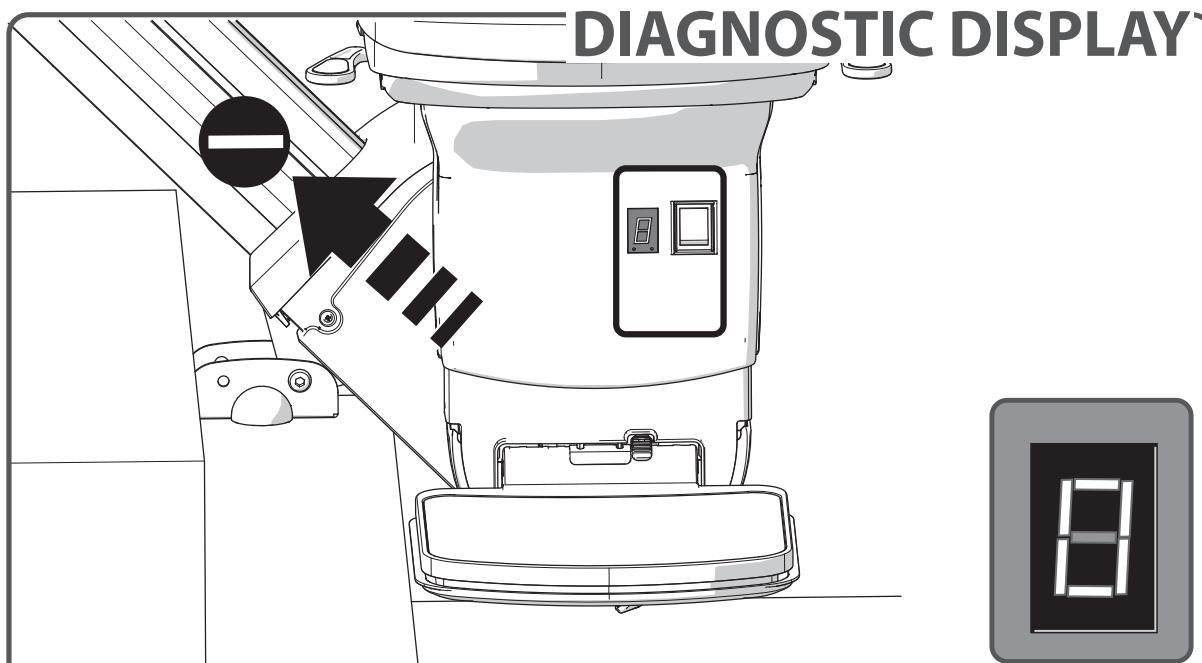
The stairlift is fitted with a diagnostic display that displays a code to help diagnose faults. Refer to APPENDIX D for an explanation of the diagnostic codes. Please inform the customer service operator of this code when reporting any fault.
